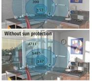
The difference in brightness between what the eye sees (30° angle) and a visual task (e.g. a sheet of paper) must be no more than a ratio of 1:3. The ratio is 1:10 for the difference between total perceived light (90° angle) and surfaces located within the field of vision (e.g. a window).
